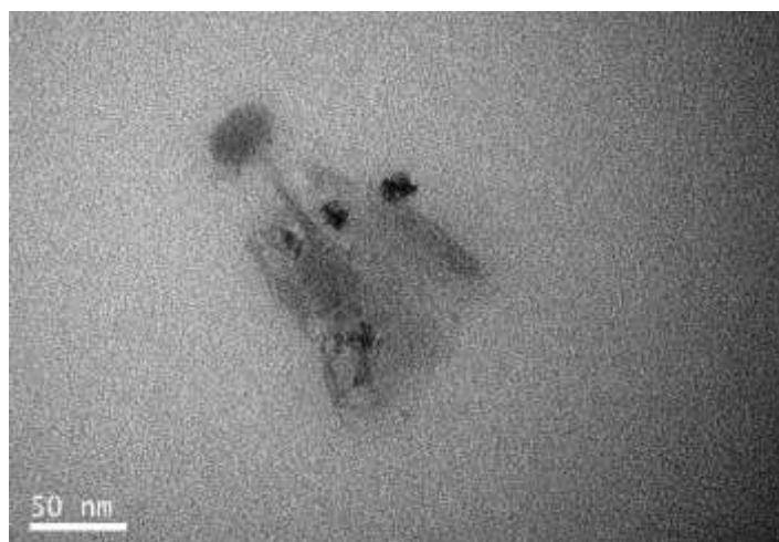
Figure 3. TEM images of GO nanoparticles (scale bar=50 nm).
